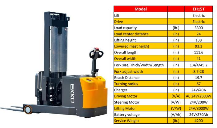
The EKKO EH15T Moving Mast Walkie Reach Truck is designed with the combination of the versatility of a forklift, reach truck and a walkie stacker. It is ideal for loading and unloading trucks, loading docks, stock rooms, manufacturing floors and warehousing.
