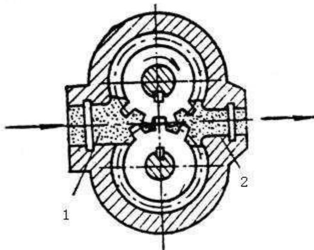
Figure 5-1 gear pump working principle diagram
