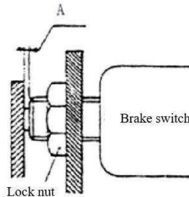
Fig.2-6 Installation of brake switch
