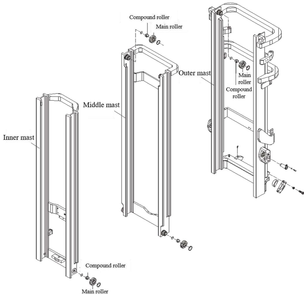
Fig. 6-13 Inner, middle and outer masts
