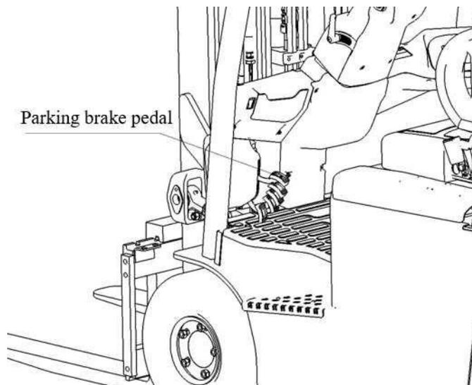
Figure 2-5 Parking brake pedal layout
