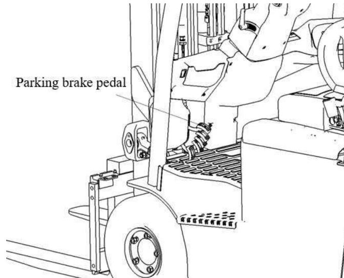
Figure 4-6 Parking brake pedal
