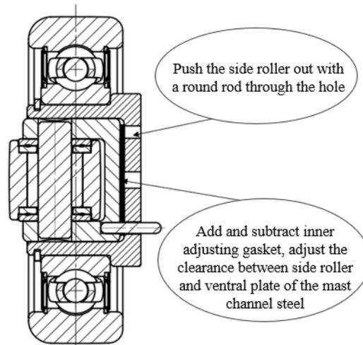
**Note: The clearance adjustment method of the side roller of the compound roller is as shown in the figure. Special gaskets are added between the side roller and the roller shaft.**
