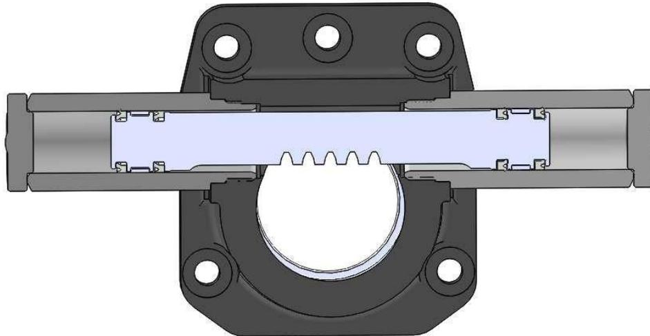
Figure 3-3 Steering cylinder
