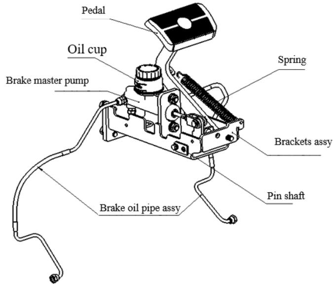
Fig.2-2 Service brake device
