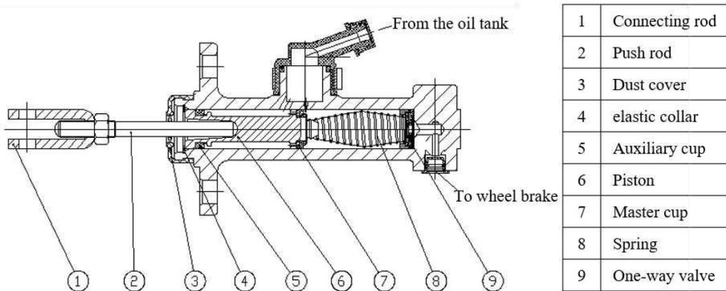
Fig.2-3 Brake master pump
