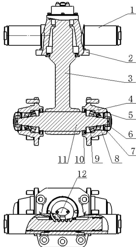
Figure 3-2 steering axle
