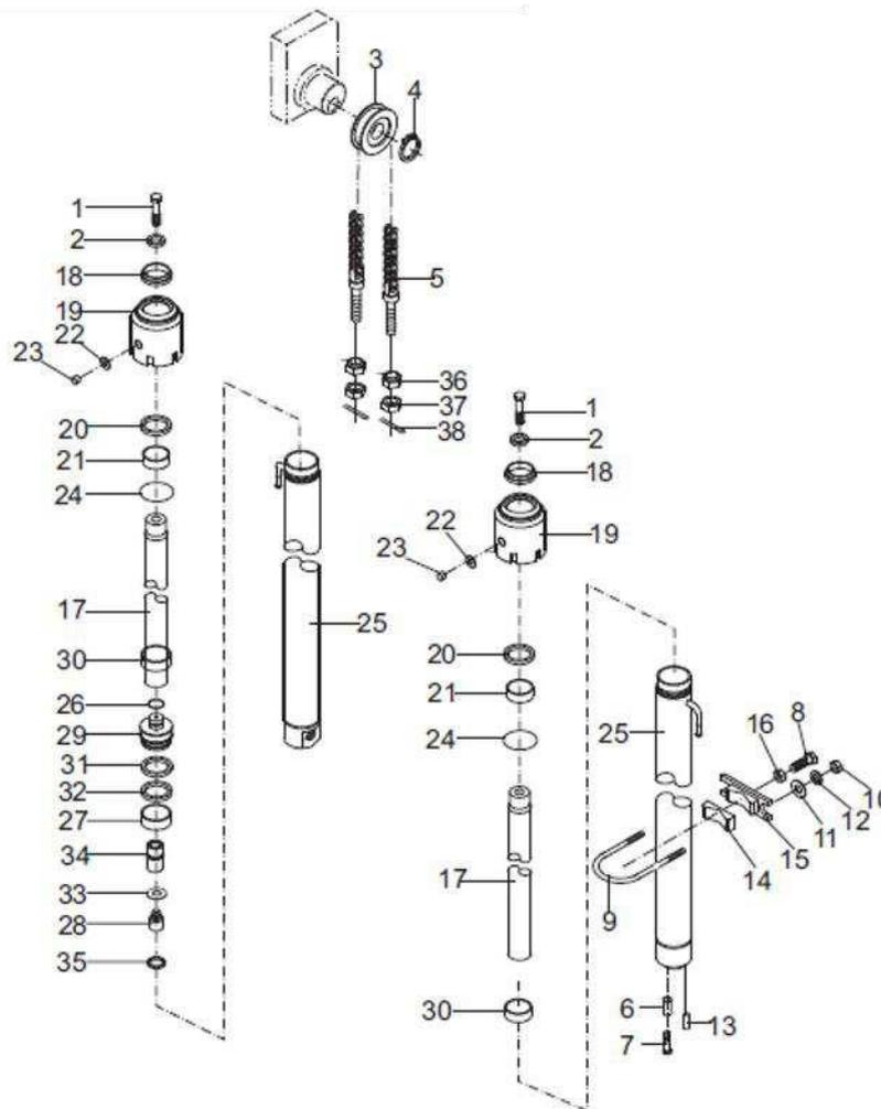
1.Bolt M16×1.5×40 2.Gasket 16 3.Chain wheel 4.Retainer ring 40 5.Chain
