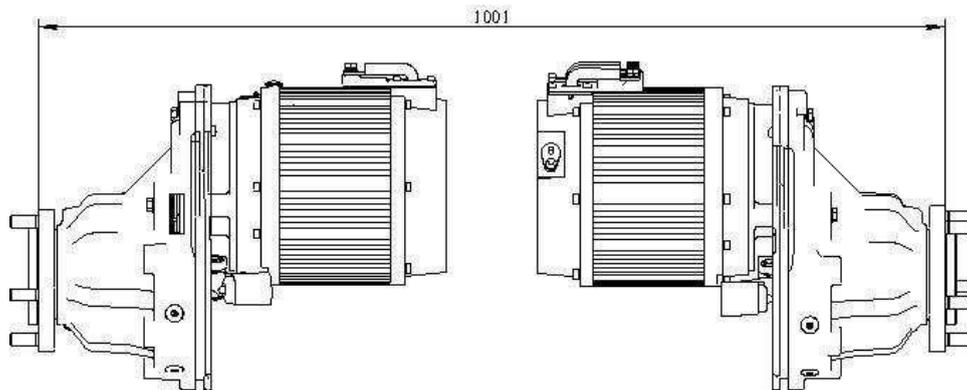
Fig.1-1 Drive axle dimensions
