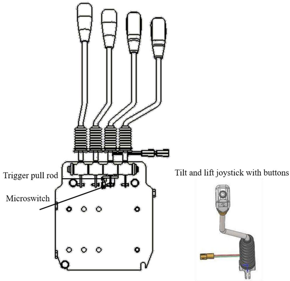
Figure 5-4 Multi-way valve control device
