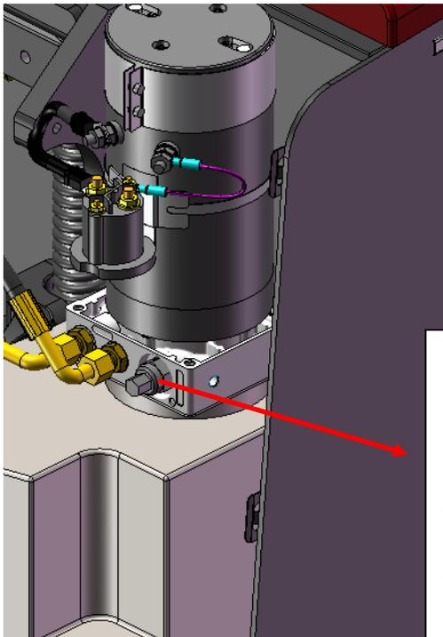
The relief value is used to adjust the oil pressure, which should be adjusted to avoid excessive pressure causing damage to the car body
