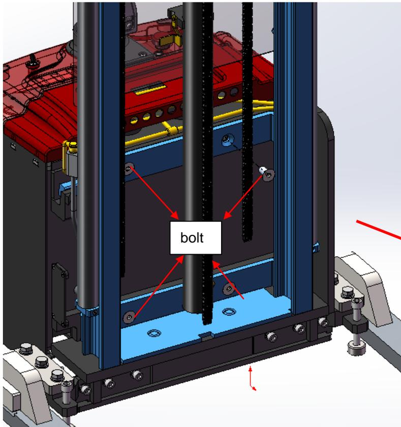
After removing the axle seat cover and bolt, the door frame can be separated from the frame. Note: the body and door frame shall be fixed with external objects during disassembly to avoid safety accidents in the process of disassembly.
