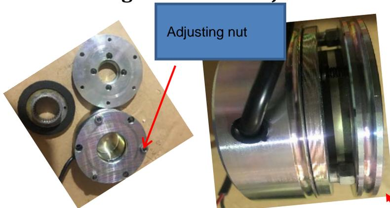
Note: electromagnetic brake can't pull properly when it is powered on in free state, it needs external force or installation to pull
