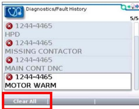
Clear All is used to Clear historical fault folders. A function key is highlighted only when there are historical failures in the historical failures folder and grayed out when there are no historical failures.
