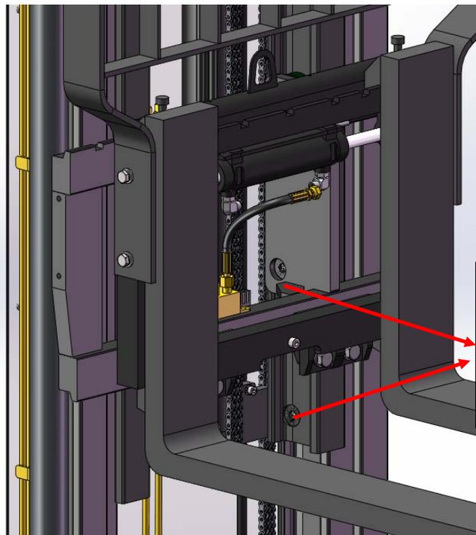
The clearance between the door frames is adjusted by adjusting the tightness of the adjusting screws
