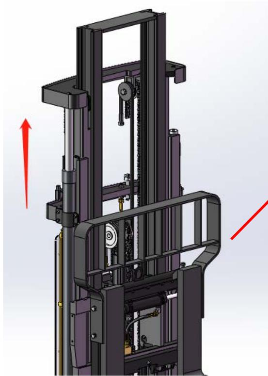
The door frame can be raised by loosening the adjusting screw
