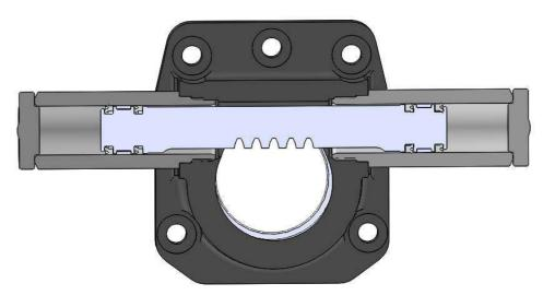
Figure 3-3 Steering cylinder
