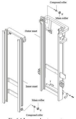
Take care when maintaining the upper combination roller of the outer mast.
