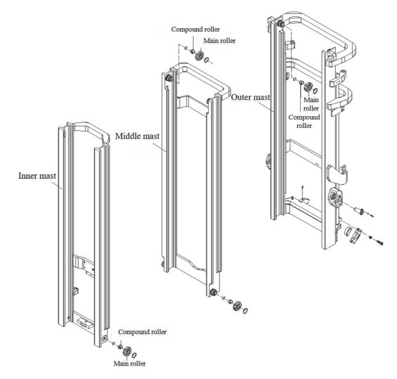
Fig. 6-13 Inner, middle and outer masts
