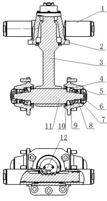
Figure 3-2 steering axle 1) steering cylinder 2) pivoting support 3) support gear shaft 4) hub 5) hub cover 6) lock nut 7) washer 8) bearing 9)bearing 10)oil seal 11)axle 12) Angle potentiometer
