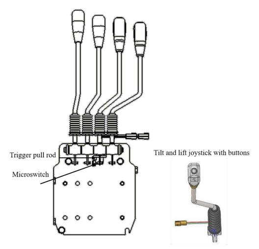
Figure 5-4 Multi-way valve control device
