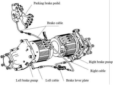
Fig. 2-4 Parking Brake Action Schematic
