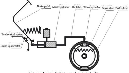
Fig. 2-1 Principle diagram of service brake
