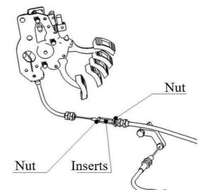
Figure 2-7 Parking Brake Cable Adjustment
