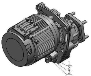
Fig.1-4 Position of brake oil port 1. Breathing cap connector 2. External braking hydraulic oil connector (M10X1) 3. External parking brake hydraulic oil connection (M10X1)
