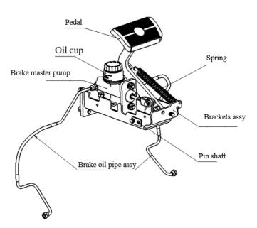
Fig.2-2 Service brake device
