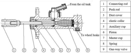
Fig.2-3 Brake master pump
