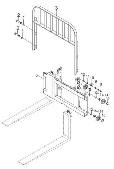
Gasket 2. Bolts 3. Load-backrest 4. Compound roller (including 13-16)
