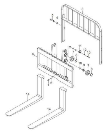
Limit screw 2. Washer 3. Load-backrest 4. Washer 5. Bolt 6. Fork carrier
