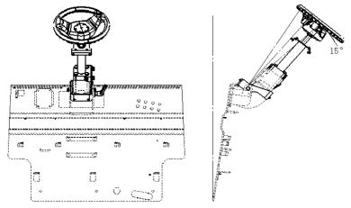
Fig.3-1 Steering control mechanism
