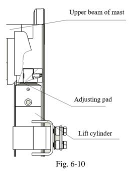
(e) When the front cylinder needs to be replaced, the fork carrier needs to be removed. The disassembling and assembling method is the same as 6.1.4(3). Remove the fork carrier as a whole, and then remove and replace the oil cylinder before lifting, as shown in the figure below.
