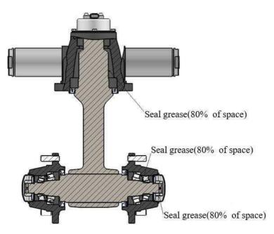
Fig. 3-5 Add grease and adjust preload
