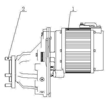
Fig.1-2 Transport of drive axle 1.Sling position 2.Wheel hub bolt
