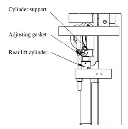
Fig. 6-17 Adjust rear lifting cylinder synchronously
