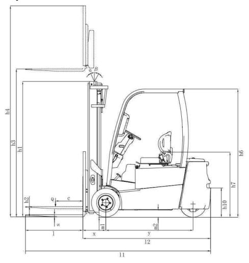
Ast: Right angle stacking aisle width a: Clearance b: Load length b12: Load width
