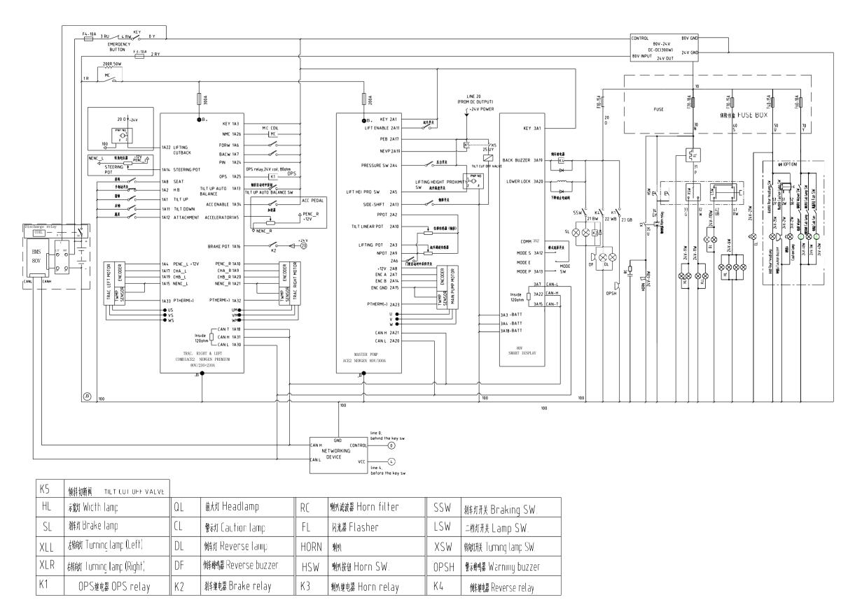
Figure 4-1c Principle diagram of electric system (ZAPI system)
