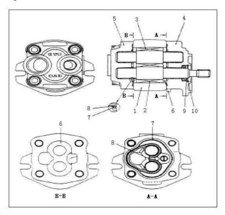
Figure 5-2 Gear pump structure outline diagram
