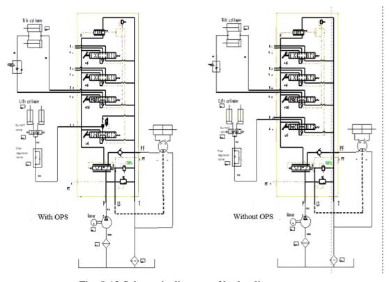
Fig. 5-12 Schematic diagram of hydraulic system (1) Hydraulic oil tank (2) Oil suction filter (3) Pump motor (4) Gear pump (5) Multi-way valve (6) Steering gear (7) Steering cylinder (8) Speed Limit Valve (9) Stop valve (10) Lifting cylinder (11) Tilt cylinder (12) Attachment cylinder (13) Return oil filter
