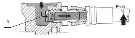
when the flow is above the specified value Fig. 5-9 Operating principle of cut-off valve
