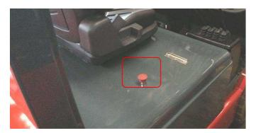
Figure 4-7 Emergency power off switch
