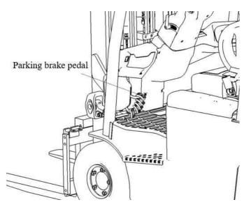
Figure 4-6 Parking brake pedal
