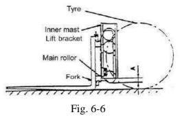
(3) Replacing rollers of the fork carrier
