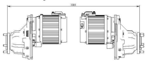
Fig.1-1 Drive axle dimensions
