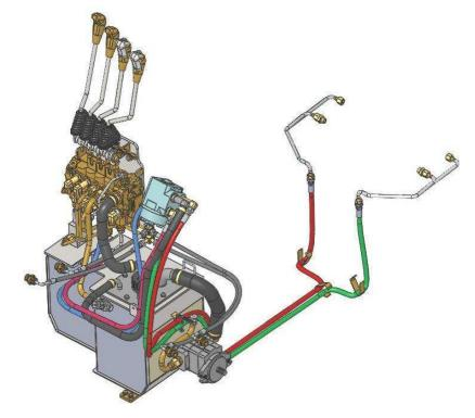
Fig. 5-13 Hydraulic Piping Diagram
