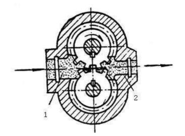
Figure 5-1 gear pump working principle diagram (1) Oil absorption cavity (2) Pressure oil cavity
