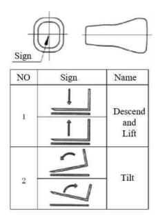
Fig. 5-5 Multi-way valve control handle identification
