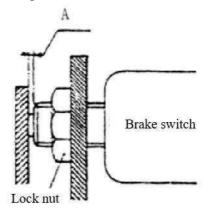
Fig.2-6 Installation of brake switch
