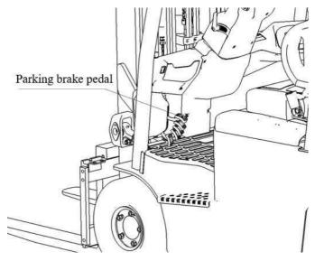
Figure 2-5 Parking brake pedal layout
