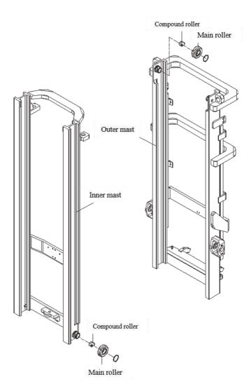
Fig. 6-7 Inner and outer mast
